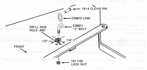
Model K41 mowers prior to serial number E53241 can be modified if interference between the mower drive belt and old style lift link exists.
