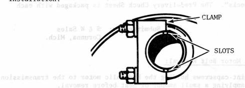
Model 446 and 448 tractors leaving the factory now have this clamp installed at the left side muffler inlet. In the near future, as soon as sufficient quantity is available it will be factory installed at both muffler inlets.
