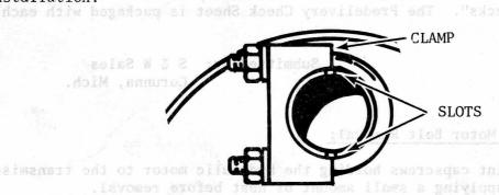
Model 446 and 448 tractors leaving the factory now have this clamp installed at the left side muffler inlet. In the near future, as soon as sufficient quantity is available it will be factory installed at both muffler inlets.
