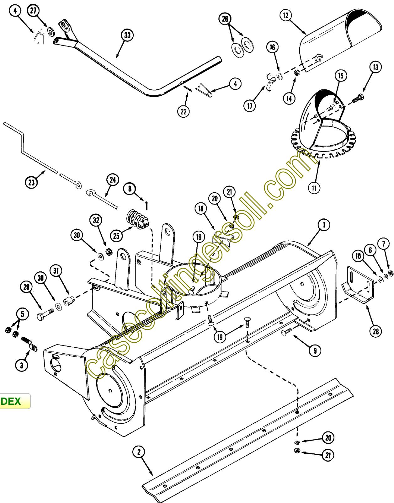
**INDEX****SB38G, SB48 SNOW BLOWER****AUGER HOUSING, CHUTE CONTROL AND LIFT ASSEMBLY**
