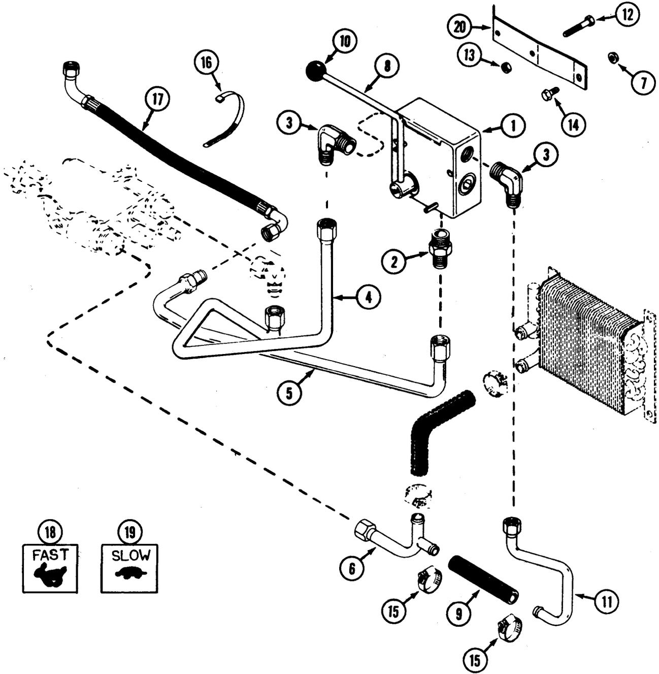
**INDEX****HFC34A FLOW CONTROL VALVE KIT**
