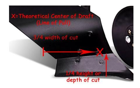
The above frontal view of a moldboard shows this point "X", an intersection of the horizontal and vertical plane. It is about 3/4 the width of the stated "width of cut" designed in a plow with each pass or furrow. And it is about 1/4th the depth of cut of the plow and is measured plumb, straight up the moldboard. The intersection of the horizontal and vertical draft planes is the exact "center of draft".
