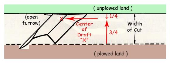
For example in the preceding illustration, if a plow is a "Twelve Inch Width of Cut" (12), then the horizontal line of draft is measured 9" from the right side of the moldboard edge. (Or, you can also measure it as a quarter the width of cut starting from the left side of the moldboard because it is harder to determine where on the moldboard wing edge where to start from).
