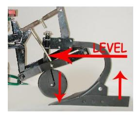
(Note: On some garden tractor plows, the plowshare, or "point" has an extended nose that dips below the landside bottom edge. This provides for additional penetration because these plows don't have the frame weight to help push the plow into the ground, once moving. As part of pre-adjustment before heading to the field, you'll have to stick a board under the landside to shim the plow bottom up enough to really level it to the driveway.)
