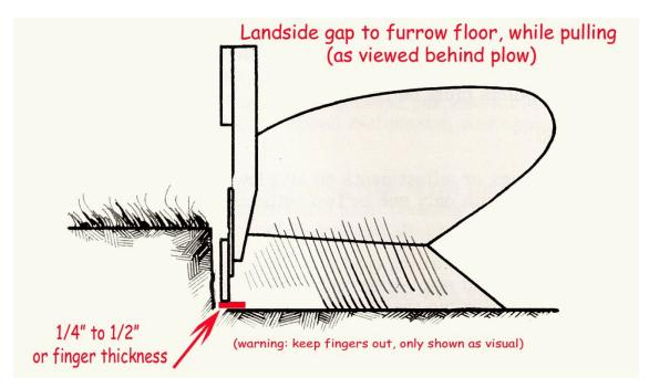
When in the field, this relationship is the same. Then once in the ground, you notice a turnbuckle either on the garden plow and/or the top link of the 3 pt. hitch. You may in some soils have to decrease the length of the turnbuckle slightly to give the plow a "nose in" attitude, or what is referred to as "suck". You can see this relationship below. The plow should pull through the ground level, but.... notice the up/down arrows are what favor "suck".
