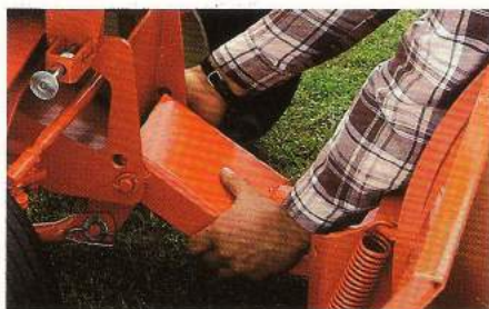
A. Simply engage the attachment bracket with alignment pins on the tractor.
