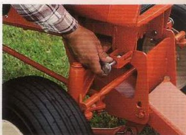
B. Release the spring loaded plunger pins to engage the holes in the mounting bracket.
