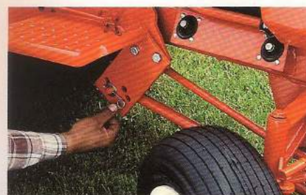
C. Secure lift arms or links on the attachment to the tractor.
