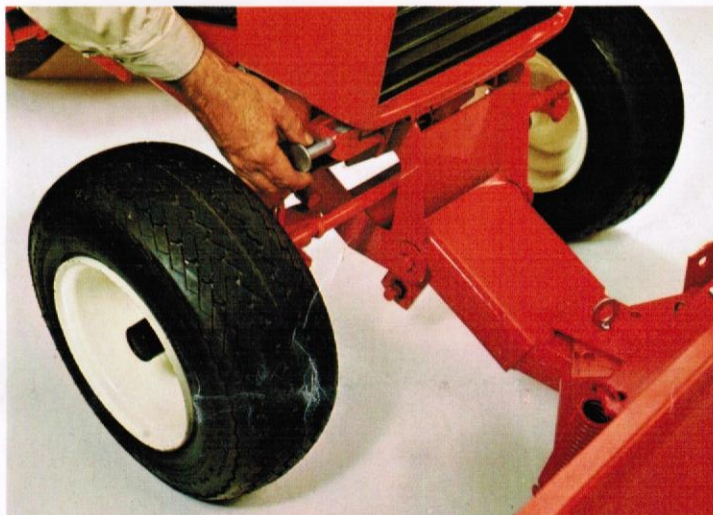
Release spring-loaded pins to lock attachment to tractor.
