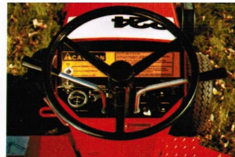
Single lever control. Hydriv lets you control both speed and direction with a single lever. Control lever is placed just below and concentric to the steering wheel.
