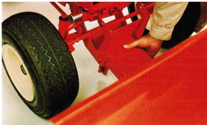
Position attachment in line with tractor mounting brackets.
