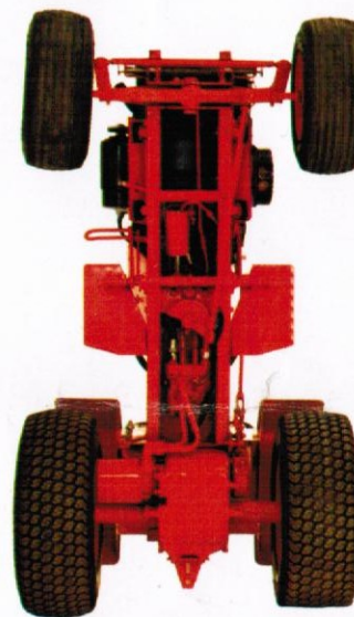
All welded twin channel frame. Designed to withstand the stress of heavy work loads. Another example of tough-job engineering that comes from just plain know-how.
