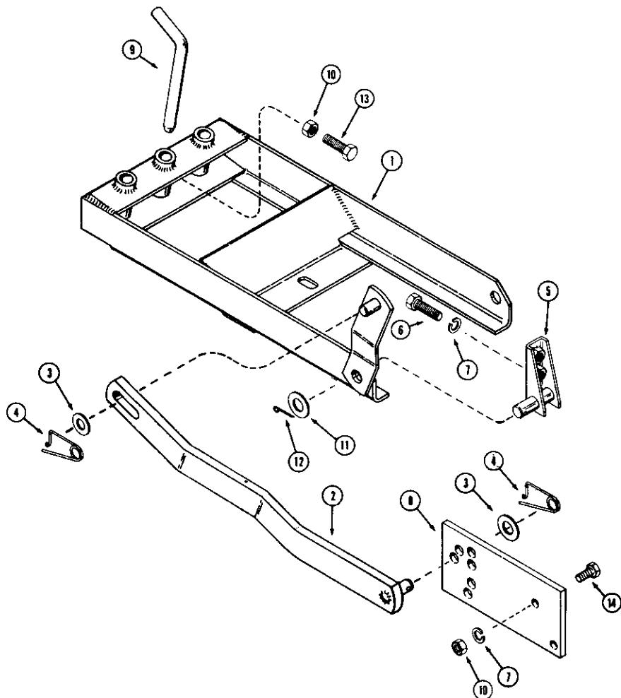
**INDEX****K22 & K22-1 SLEEVE HITCH (Used on 3000 Series)
