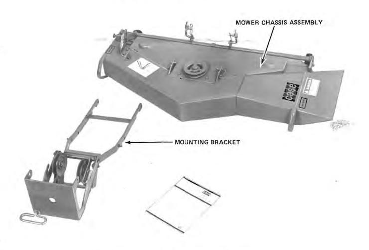
FIGURE 12 MODEL K44 ROTARY MOWER - DISASSEMBLED
