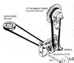
1) WIND KEY CLOCKWISE BY HAND AS FAR AS POSSIBLE AND PLACE ATTACHMENT DRIVE IN ENGAGEMENT POSITION
