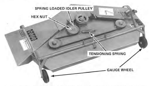
FIGURE 8 K44 MOWER WITH BELT GUARD REMOVED FOR A CLEAR VIEW
