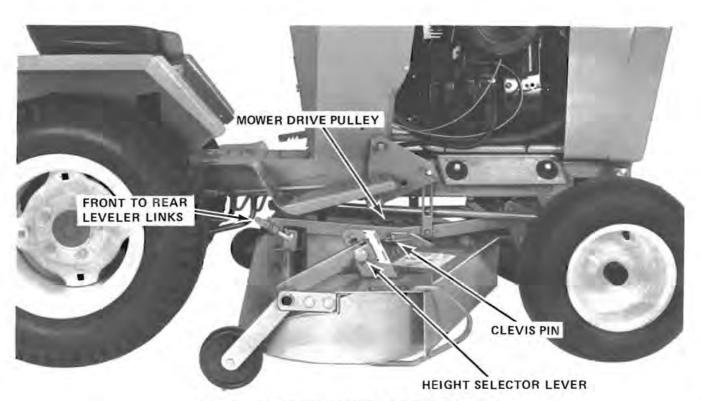
FIGURE 16 MOUNTING THE K44 MOWER CHASSIS
