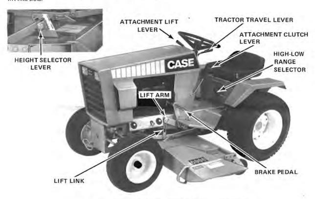
FIGURE 1 (MODEL 222 WITH MODEL K44 ROTARY MOWER)
