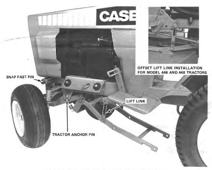
FIGURE 15 MOUNTING THE K44 MOWER MOUNTING BRACKET
