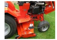
Step 3. Disconnect mounting (Mule) bracket by releasing Snap-Fast pins while deck is suspended by Lift Links.
