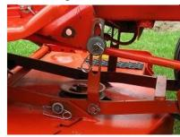
Step 5. Shut off engine and disconnect Right and Left Lift Links.
