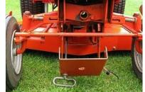
Step 4. Lower deck to ground by completely lowering lift arms.
