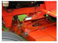
Step 8. Insert Anchor Rods through deck axle on both sides and into ground to hold deck from sliding on grass.
