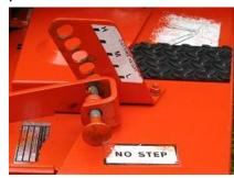
Step 7. Place Deck Ramps behind front tires and against front of deck on both sides.
